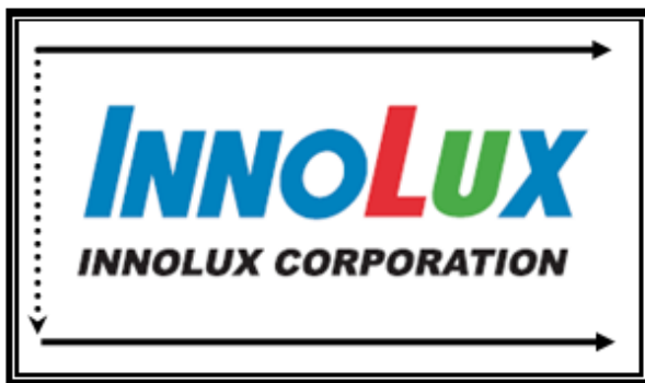
RPFI = Low/floating; normal display (default)
