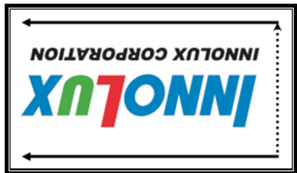
RPFI = high: display with 180degree rotation
