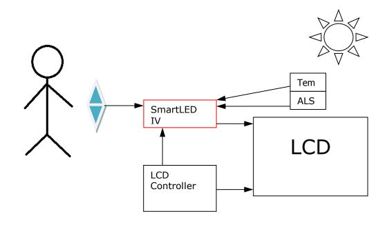
Figure-1: Overview of SmartLED-IV usage (ALS = ambient light sensor)
